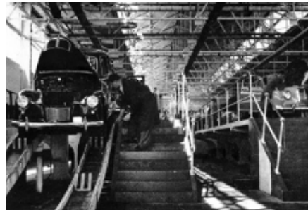
fig. 12.61. An example of Final inspection area in an Austin Automobile assembly line (1950s). Cars received an inspection and final polishing before went to test drive.
