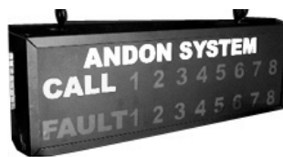
fig. 12.62. Andon system to communicate problems in machines
