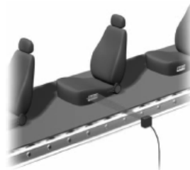
fig. 12.56. Barcode Reader, a poka-yoke system used in automobile industry to check completeness of the components need to be mounted to the passenger seats (belt buckle, side air bag, passenger check module, seat weight sensor and seat position sensor)
